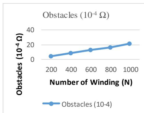
**Figure 6.** The graph of the variation in the number of circumferences with the obtained resistance
