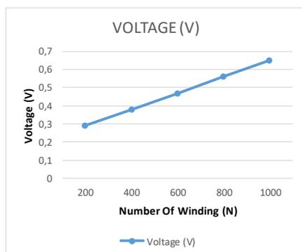
**Figure 4.** Graphs of the data variation in the number of turns with the resulting voltage
