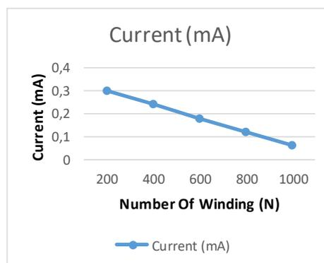
**Figure 5.** Graph of the data variations of the number of winding with the current
