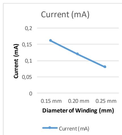
**Figure 8.** Graphs of variation of circumferential diameter data with the resulting current
