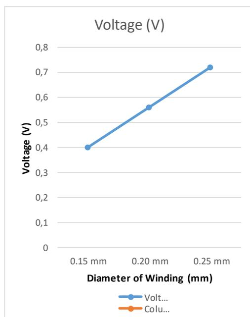
**Figure 7.** Graphs of variation of circumferential diameter data with the resulting voltage
