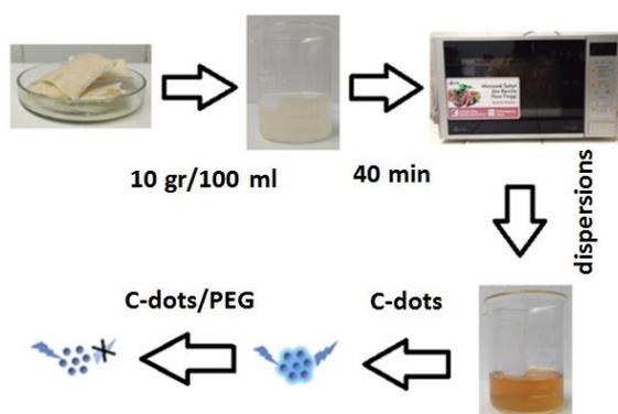
**Figure 1.** Scheme of synthesis and passivated of C-dots
