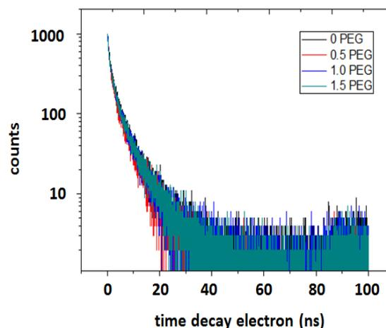
**Figure 4.** Time-resolved photoluminescence spectra of colloidal C-dots
