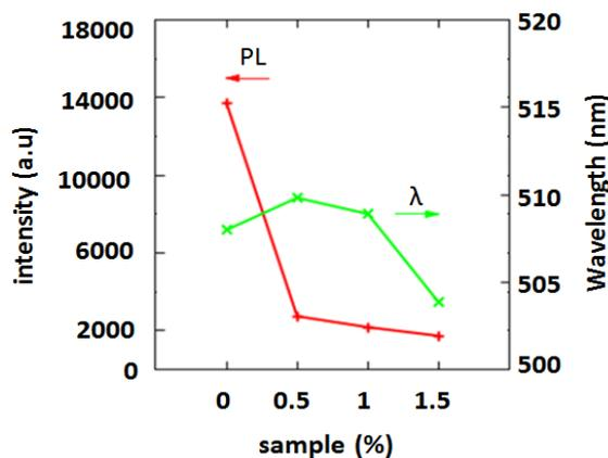
**Figure 3.** Curve relationship between peak PL intensity and wavelength of C-dots
