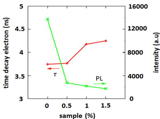
**Figure 5.** The relationship between PL intensity and Electron time decay C-dots
