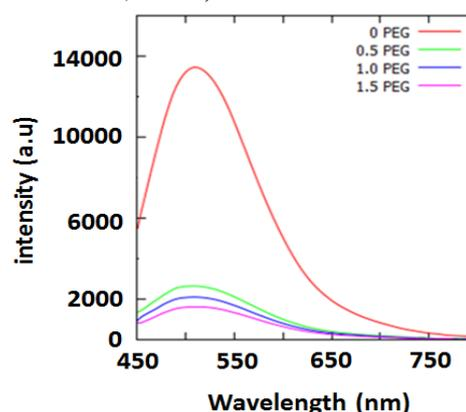
**Figure 2.** Photoluminescence spectra of colloidal C-dots
