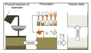
**Figure 4.** Wastewater purification steps, ie filtration, decantation, and coagulation (Source: Néel et al., 2015)
