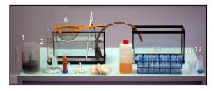
**Figure 3.** Setting tools and practicum materials: (1) 500 mL cup glass containing sediment; (2) water; (3) clay; (4) gravel; (5) polystyrene sticks; (6) strainers; (7) stirrer; (8) aquarium pumps; (9) FeCl3 0.1 M; (10) reaction tube shelf; (11) 50 mL cup glass; (12) electrolyte solution; and two aquariums (Source: Néel et al., 2015)
