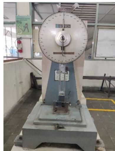
Gambar 3 Impact Test GOTECH Model KT-7045.
