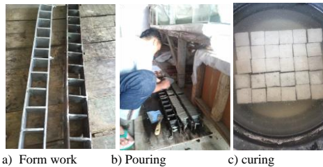
Figure 2. Pouring and curing specimen
