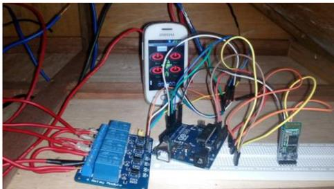
Gambar 4. Rangkaian arduino, relay, *bluetooth*, android
