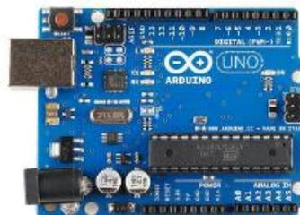
Gambar 1. Board Arduino Uno
