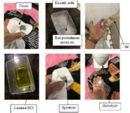
Gambar 3. *Surface Preparation* Spesimen **Proses *Hot Dipping Galvanizing***
