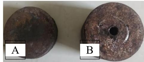
Gambar 4. *Pressing* alat tambal ban: (A) *Pressing non valve* (B) *Pressing valve*
