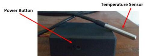
Gambar 1. Modul Transmitter
